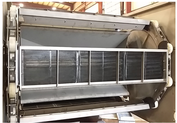
Heavy duty carrier chain, baskets and drive sprockets
